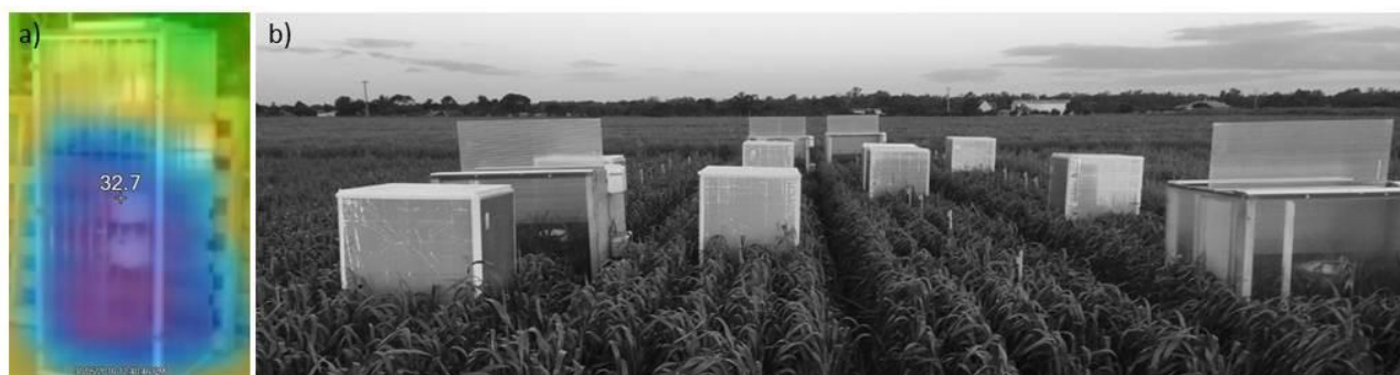
Figure 1. Frost chambers a) Performance testing using visual IR thermometer, Fluke VT02 (temperature at 32.7 °F (0°C)) and b) Simulated frost being applied to wheat to determine impact on yield and ultimately the link between frost induced sterility and proximal sensor response.
