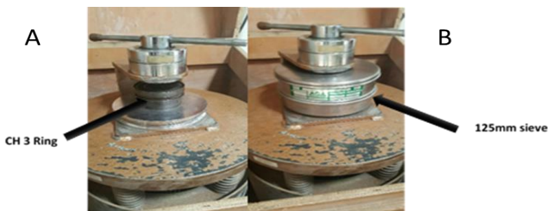
Figure 1. (A) The RockLabs ring miller (0.18KW) New Zealand with CH3 ring for milling and (B) The RockLabs ring miller (0.18KW) New Zealand with 125mm sieve of ABICHEM Test Sieve BS 410 for the shaking.
